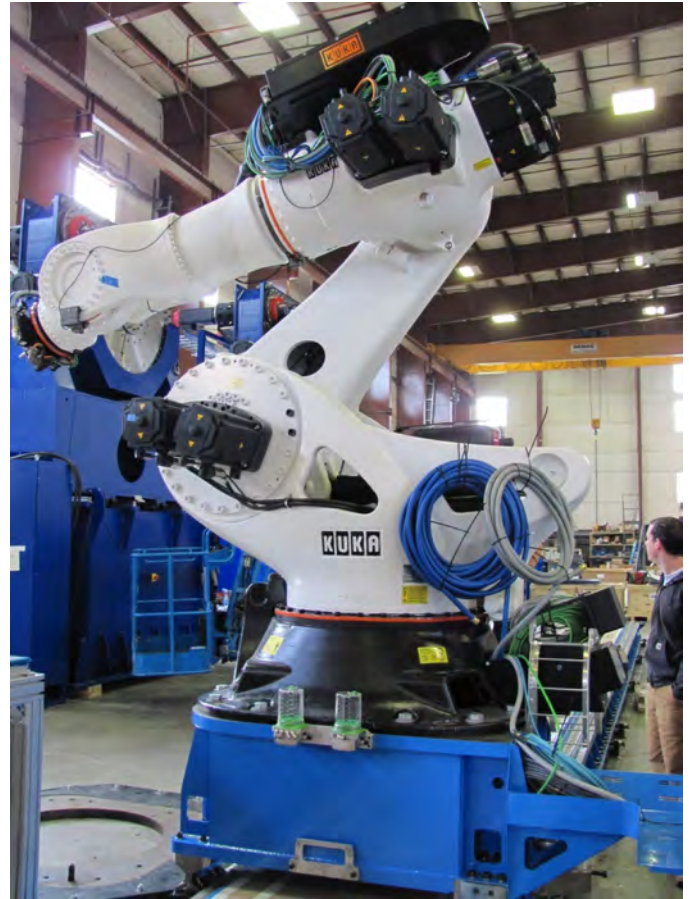
Figure 2. Accurate Robot (KUKA KR1000L750) with optical scale secondary feedback installed.
