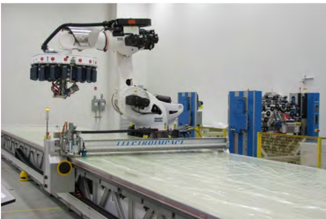
Figure 6. Accurate robot AFP system integrated with a large vacuum table, CNC controlled ultrasonic ply cutting gantry, and AFP head transfer stands.
