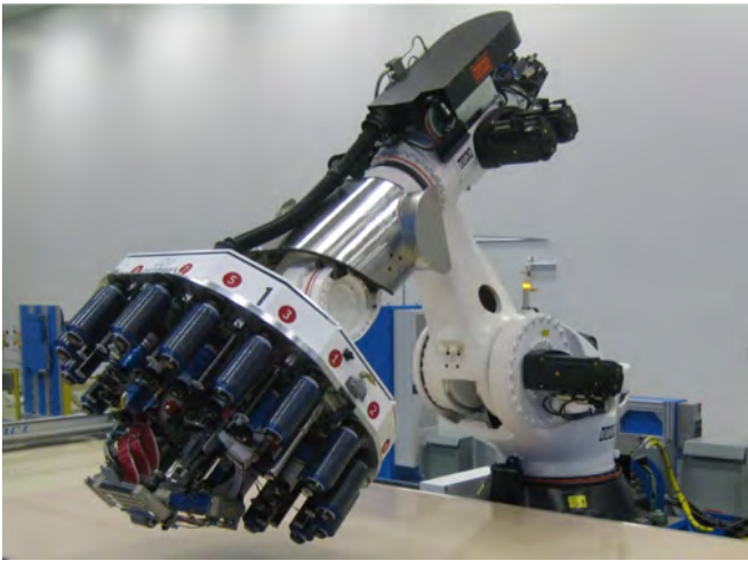
Figure 5. Accurate robot with a modular AFP head.
