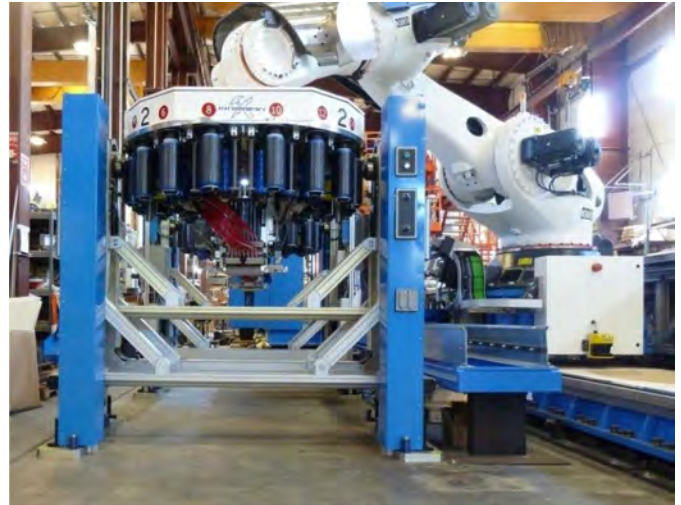
Figure 7. AFP head interfacing with a head transfer stand.
