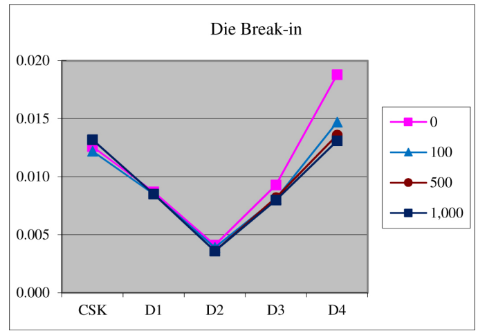
Figure 6. Break-in Period showing a reduction in D4 interference over the first 1000 cycles of use.
